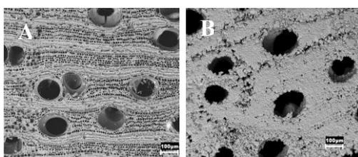
Figure 1.- SEM micrographs of A) sapelli carbon preform and B) sapelli BioSiC
